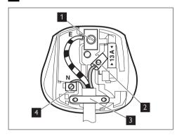
The wire coloured green and yellow must be connected to the terminal marked with the letter «E» or by the earth symbol  $\perp$  or coloured green and yellow.
